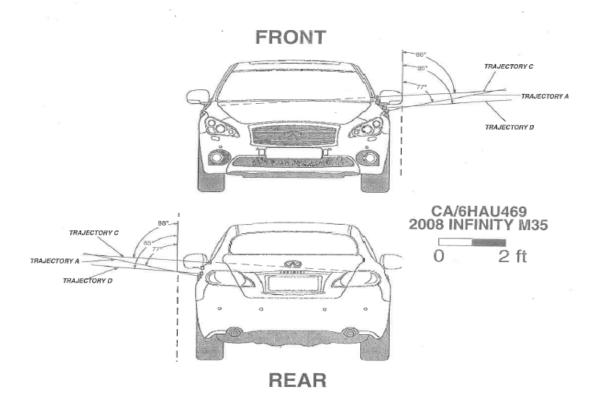
Figure 3: Bullet trajectory analysis. (Source: CSI)
